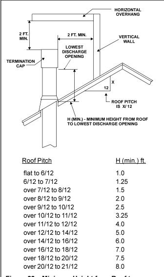
Figure 22. Minimum Height from Roof to Lowest Discharge Opening
